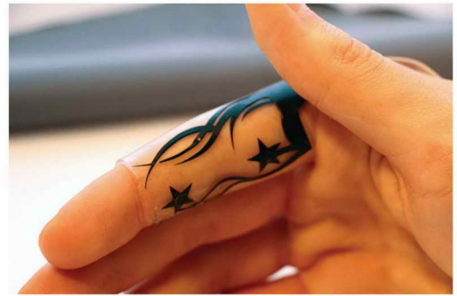
Figure 3. Aesthetic on-skin devices. The iSkin touch sensor is thin and stretchable. Using digital fabrication, it can be customized to fit the user's aesthetic preferences and individual proportions so it can be worn at various locations on the body.
